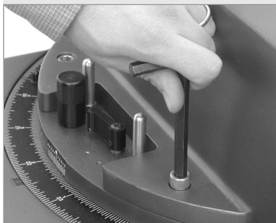
Fig. 51: Bolt the fork to the drive base.
