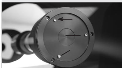
Fig. 59: Insert the included hex wrench into the slots in the plate of secondary mirror housing to access the collimation screws (14" model only).
