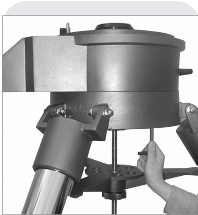
Fig. 50: Attach the drive base to the tripod.
