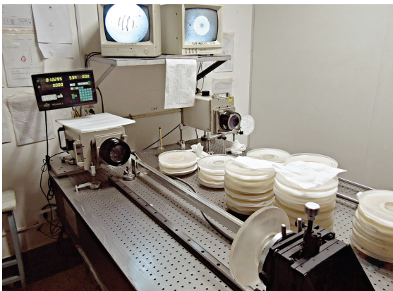
FIGURE 10. We test all of our primary mirrors on an optical bench by means of laser interferometry. In the picture, stacks of polished primary mirrors await testing.
