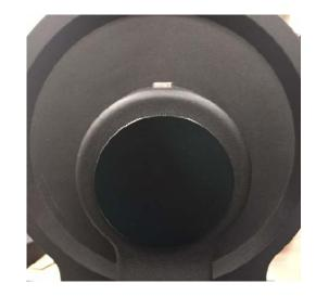
4. Remove counterweight shaft house by unscrewing three screws (one socket screw on top and two set screws on the side).
