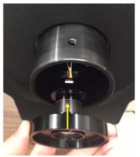
6. Back out two set screw to make sure they do not stick out of the outside ring. Psuh the iPolar into the RA axle. Tighten two set screws on iPolar CEM120 adapter to secure the iPolar inside the RA axle. Do not over tighten the screws.
