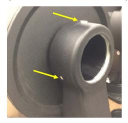
5. Plug the 4 wire cable to the iPolar. Insert it into the CEM120 RA axle. You may use a wire to pull the cable to the rear of the RA axle.
