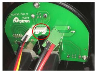
If your CMS\_D has an USB plug for the iPolar, please contact iOptron for a modified one.
