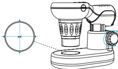
Place the object to be observed in the center of the observation area of the microscope table. Adjust the table height and observe the changes on the screen. When the picture becomes clear, you can take pictures or videos.
