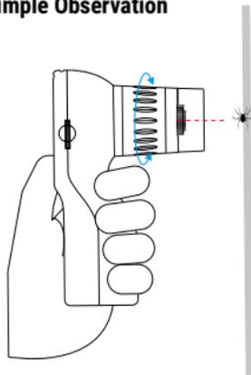
Long press the power button (12) to activate the screen. Place the object to be observed at the center of the screen. Short press the LEFT (11) or RIGHT button (14) to adjust the zoom level and use the focussing wheel (16) to adjust picture clarity.
