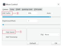
3.4 The longer the exposure time is, the lower the FPS will be. FPS indicates the frequency (rate) at which consecutive images (frames) are captured or displayed per second. Given the resolution is unchanged, frame rate = 1s/exposure time (s). If the exposure time is 1s, then the fps in this case is 1fps.
