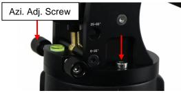
Level the mount by adjusting the tripod legs. Use the build-in Bubble Level Indicator or an external leveler for this purpose.
