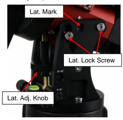
Two latitude ranges, 0~35° and 25~60°, can be set up for the mount head. To change the latitude range from one to the other, **both** the Latitude Position Bolt and the Latitude Locking Screws need to be moved to the correct locations (see photos below).
