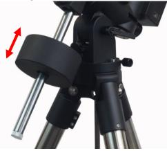
[TIP: CEM26 comes with a 10.4 lbs (4.7 kg) CW, which should be sufficient for an 8" scope with total payloads up to about 13 lbs (6kg). Use extra CW or CW Extension Bar to balance higher payloads.]
