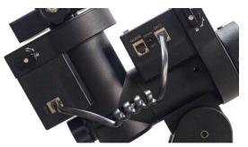
Connect the Go2Nova<sup>®</sup> 8409 Hand Controller to the **HBX** port on the main unit. Plug in a 12V DC power supply to the **DC12V IN** socket next to the **HBX** port, not the DC12V OUT next to GUIDE port.
