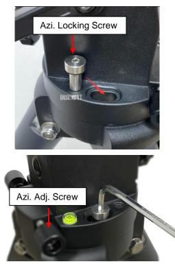
Level the mount by adjusting the tripod legs. Use the build-in Bubble Level Indicator or an external leveler for this purpose.
