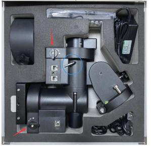
If the mount has a AccuAlign<sup>TM</sup> optical pola scope, the Allen wrench will **NOT** be inserted here.
