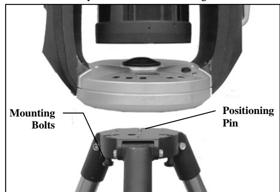
Figure 3-2 Mounting the Telescope
