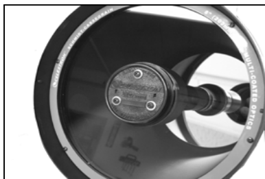
Figure 9-1 Collimation Adjustment Screws
