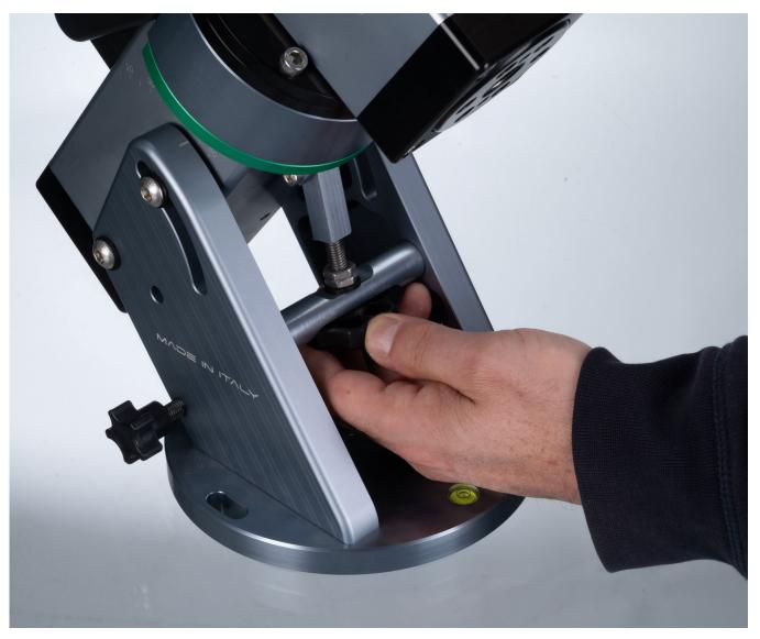
NOTE: The latitude fine adjustment must be accomplished with the four fixing lateral brackets bolts loosened. When the latitude has been set, they must be tightened again.
