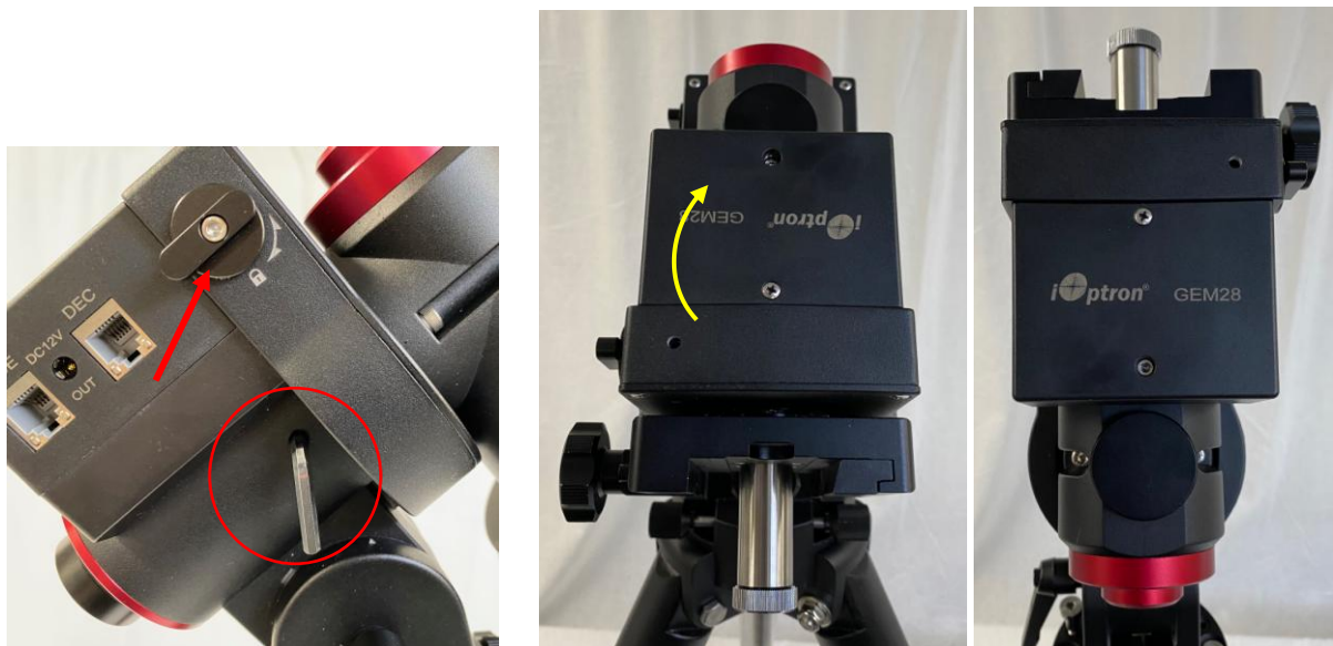
Figure 10. Rotating GEM28 mount head upward
