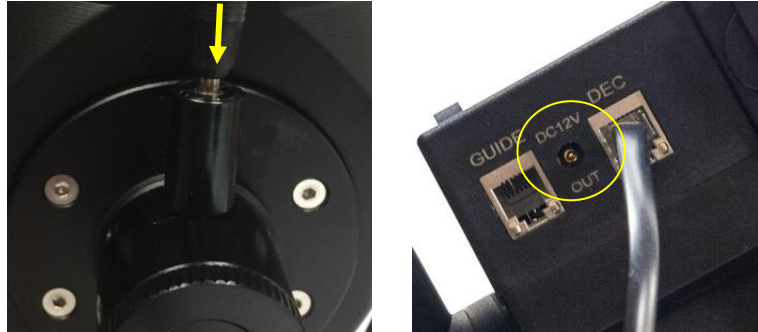
Figure 22. Connect polar scope LED
