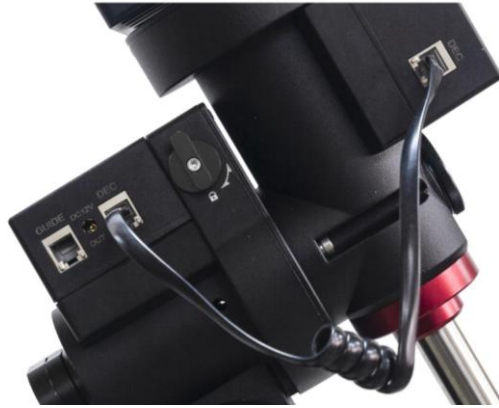
Figure 18. Connect DEC cable
