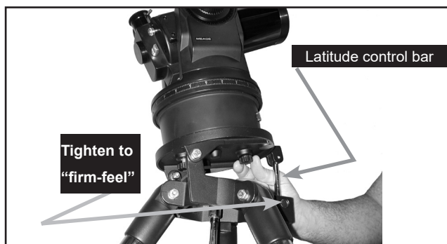
Figure 26: Attach Telescope to Tripod
