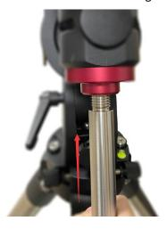
6. <u>Install counterweight</u>: Before putting on CW, make sure the mount is at its zero position, i.e., CW shaft points to the ground. **Insert Allen wrench to lock the RA axle** and disengage the R.A. Gear Switch to set the R.A. axis free before loading the CW. Remove the CW
