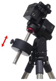
[TIP: GEM28 comes with a 10.4 lbs (4.7 kg) CW, which should be sufficient for an 8" scope with total payloads up to about 13 lbs (6kg). Use extra CW or CW Extension Bar to balance higher payloads.]
