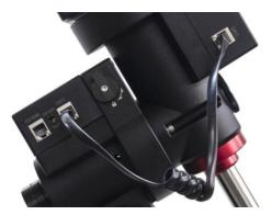
Connect the Go2Nova<sup>®</sup> 8409 Hand Controller to the **HBX** port on the main unit. Plug in a 12V DC power supply to the **DC12V IN** socket next to the **HBX** port.
