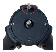
3. Attach mount head: Before put the mount onto the tripod, make sure the RA gear switch is at lock position to prevent mount head free swing by accident! Retract the 2x Azimuth (Azi) Adjustment Screws from both sides to leave ample space for the alignment peg to be fitted in between the 2x Azi
