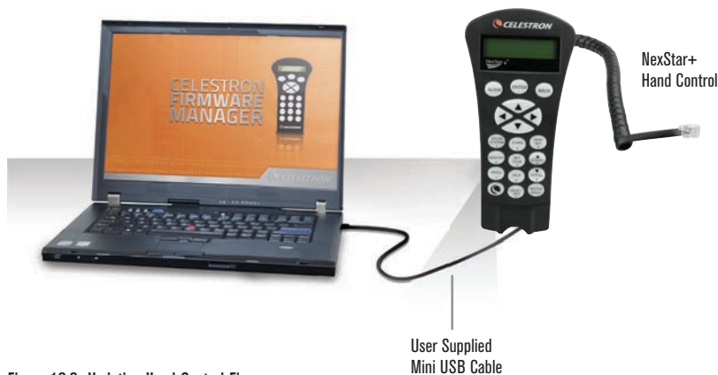
Figure 12.2 Updating Hand Control Firmware
