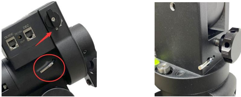
Figure 12. Allen wrench to lock the RA axle and storage
