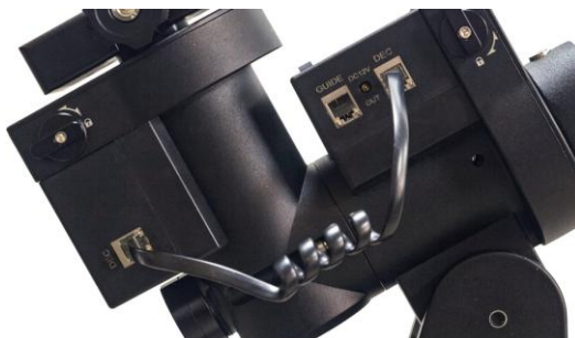
Figure 18. Connect DEC cable
