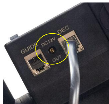
Figure 22. Connect polar scope LED
