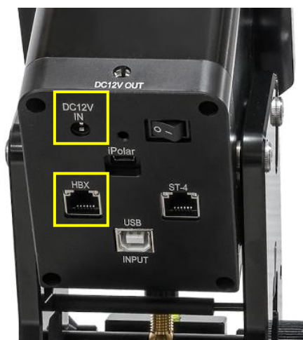
Figure 17. DC power and HBX ports
