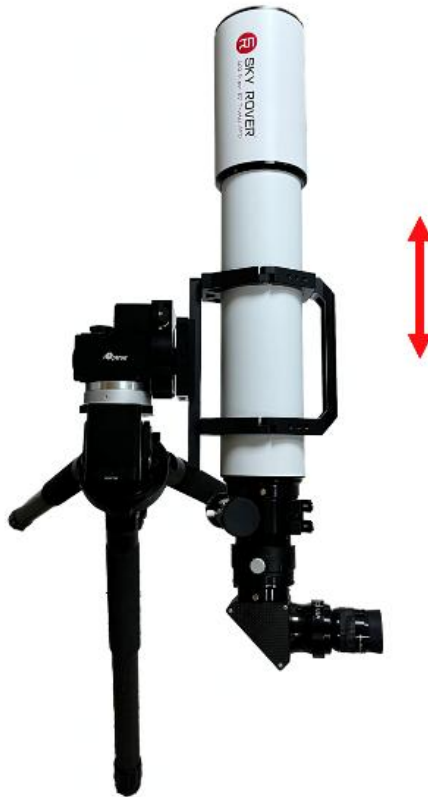
Figure 18 Balance the mount in DEC
