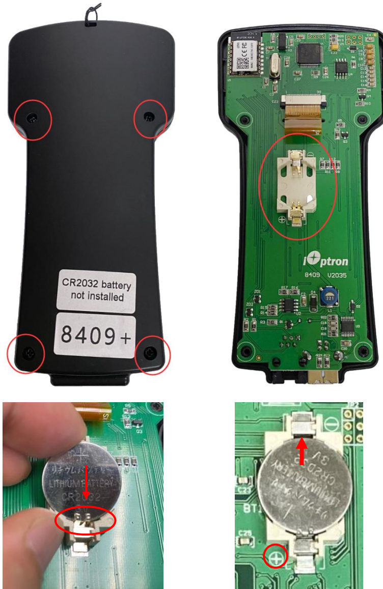
Figure 8. Install a CR2032 battery
