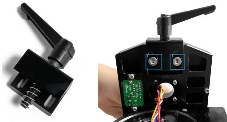
Figure 15. Convert dovetail saddle to accept a Losmandy-D plate (2) (4) Put the dovetail saddle back and retighten the four yellow circled screws. Here is a dovetail saddle that can receive a Losmandy-D dovetail bar.
