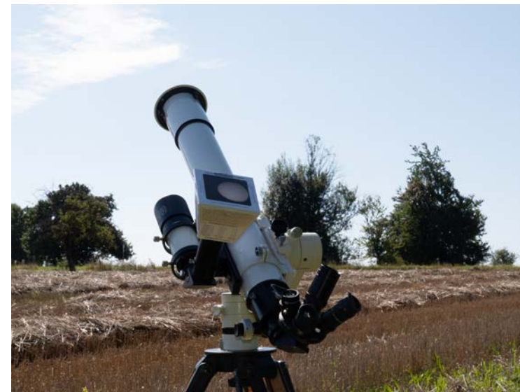
Observing the Sun with a telescope with ASTF-front filter on a simple mount. The Solar Projection Screen is mounted on a VarioFinder to control the tracking, e.g. during public events.
